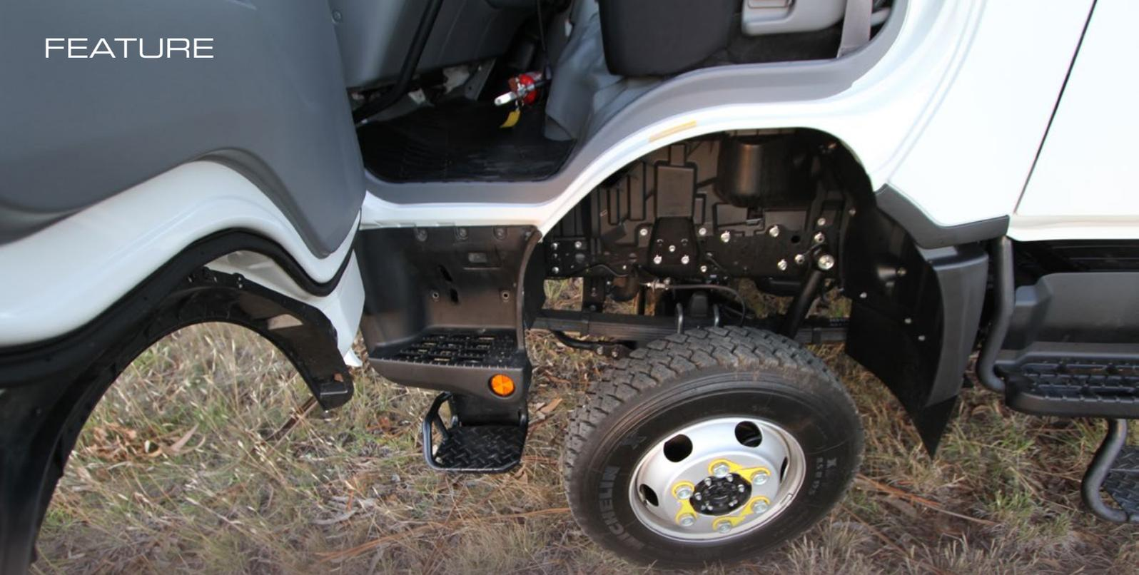
The Hino 300 Series 4x4 is available in single-cab for three people, and a crew-cab configuration as tested that can take up to seven. However, with the multi-leaf spring suspension the ride is noticeably stiffer than a standard 4x2.
