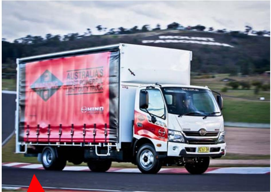
**Hino has to convince its customers that safety is a first consideration in purchase selection. This should be a prime factor in the decision making of any company operating light trucks. With ABS and vehicle stability control coupled with disc brakes the Hino 300 Series is an imposing package.**
